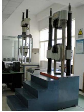
Tensile Testing Machine for PC Strand.
