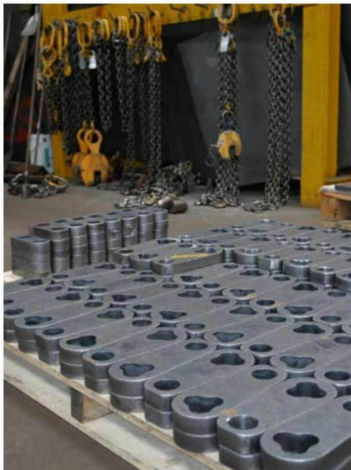
Profile cut plate parts ready for dispatch from Profile Cutting Services - a wholly owned subsidiary.
